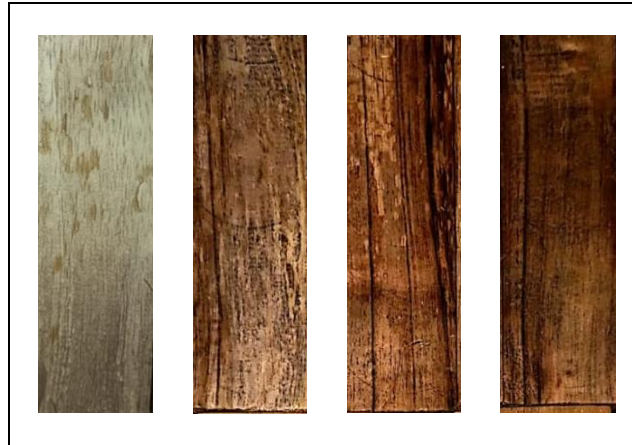
Figure 5. The Appearance of Sengon Wood Before and after Oil Heat Treatment. The Results, from Left to Right, are Control, 170°C, 190°C, and 210°C.
