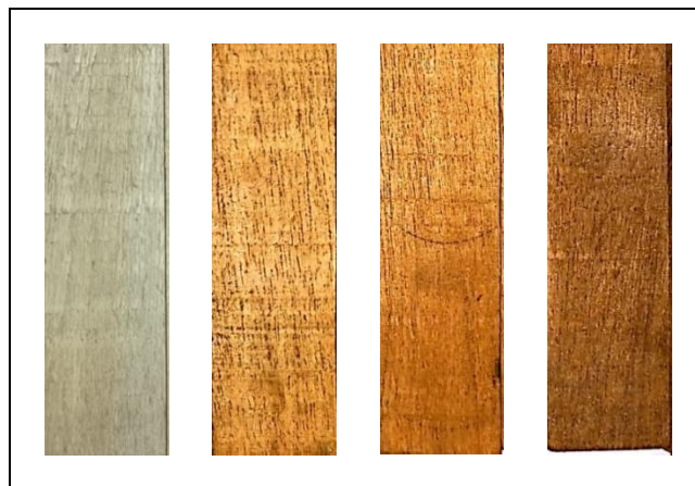
Figure 6. The Appearance of Jabon Wood before and after Oil Heat Treatment. The Results, from Left to Right, are Control, 170°C, 190°C, and 210°C.
